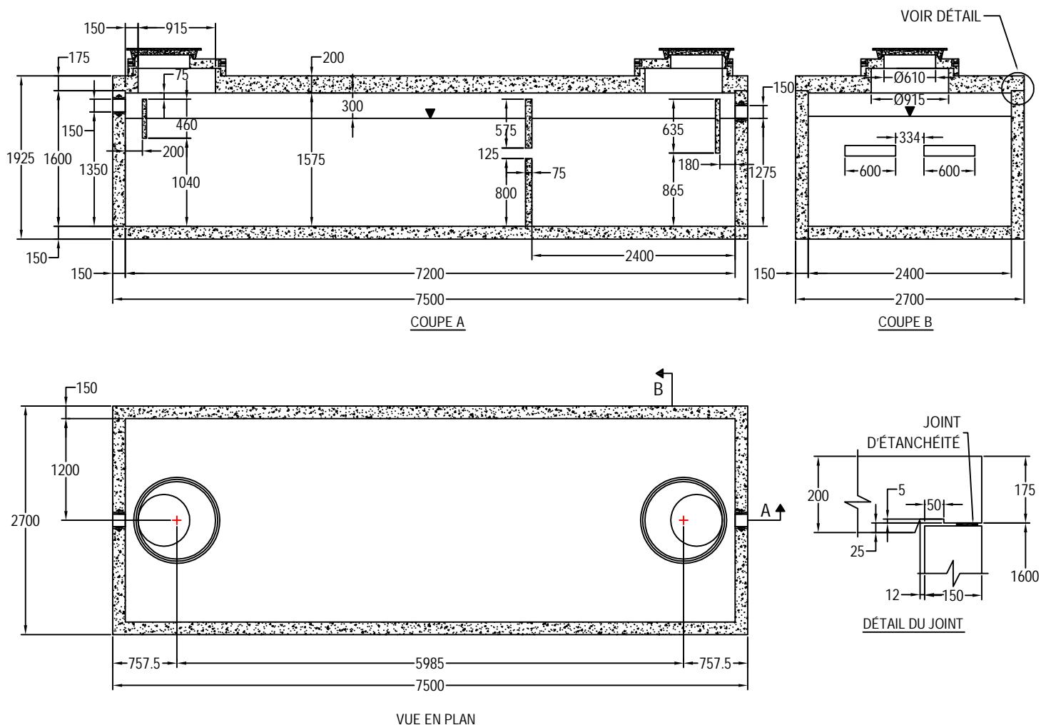
N.B.: REMBLAI MAXIMAL 900 mm.
