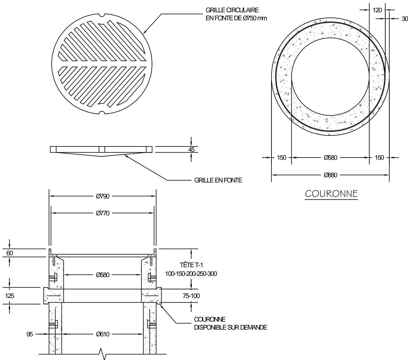
LA TÊTE T-1 DOIT ÊTRE INSTALLÉE SUR UN ANNEAU DE TYPE "D" OU "E" OU UNE COURRONNE.
