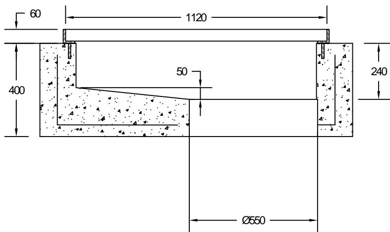
LA TÊTE RECTANGULAIRE 470 x 1030 DOIT ÊTRE INSTALLÉE SUR UNE SECTION "D" OU "E".
