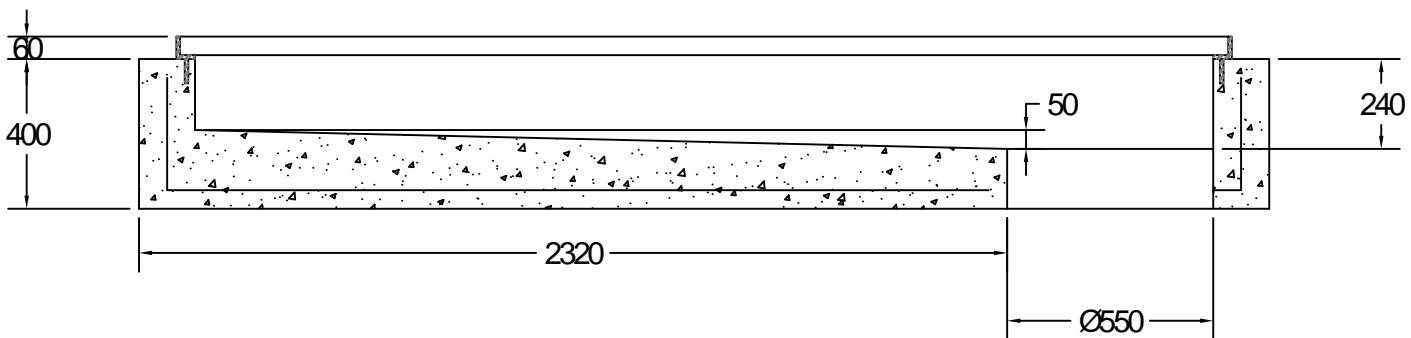
LA TÊTE RECTANGULAIRE 490 x 2720 DOIT ÊTRE INSTALLÉE SUR UN ANNEAU DE TYPE "D" OU "E".
