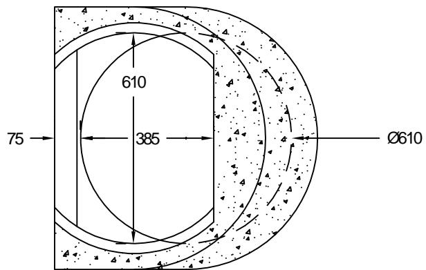
LA TÊTE T-15A DOIT ÊTRE INSTALLÉE SUR UNE SECTION "D" OU "E"..
