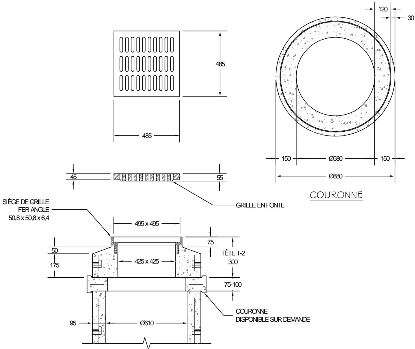
LA TÊTE T-2 DOIT ÊTRE INSTALLÉE SUR UN ANNEAU DE TYPE "D" OU
