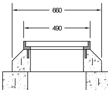
LA TÊTE T-3 DOIT ÊTRE INSTALLÉE SUR UN BOURRELET.
